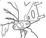
Use Correct Exhaust Gaskets
